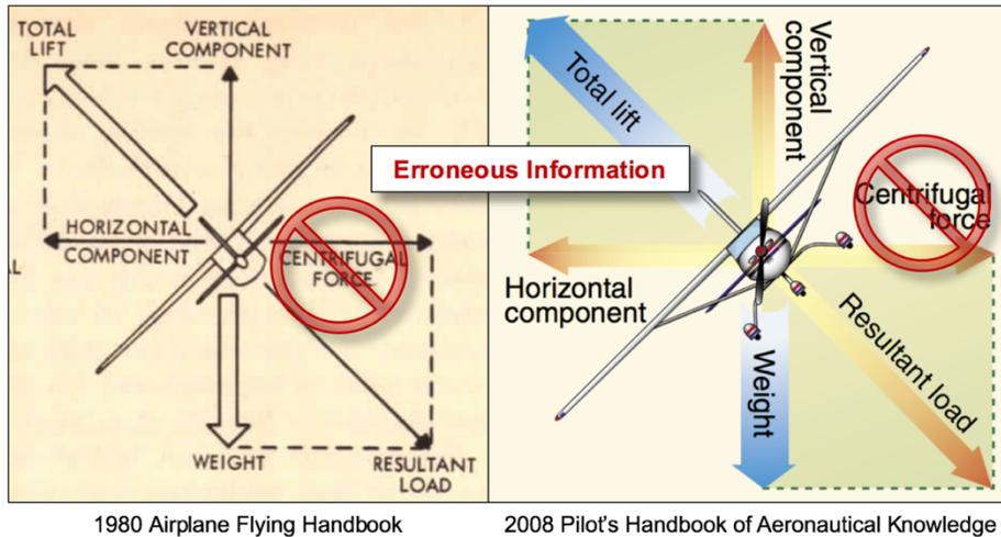
To answer the obligatory question “what turns an airplane,” pilots memorize “the horizontal component of lift.” That is an acceptable answer provided you are talking only about level turns, but airplanes are capable of climbing and descending turns, too. In the broadest sense, turns can occur in the horizontal, oblique, or vertical planes, and they occur for one simple reason: excess Lift (or alternatively, excess G).<sup>26</sup>
